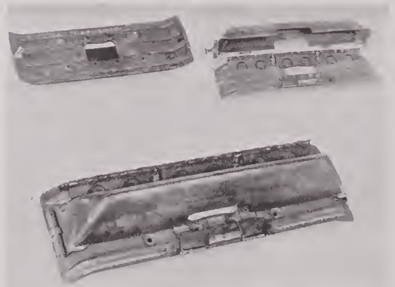
FIGURE 16. Inner side of grouser plate (top left), grouser and grouser plate (top right), and assembled unit developed for T-15 Weasel.
